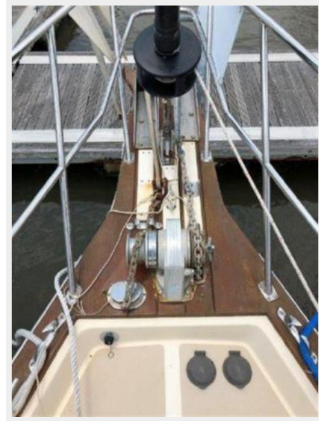
Three anchors, two rollers and a windlass
