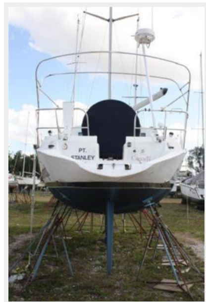
Transom/Swim Platform Extension from Astern
