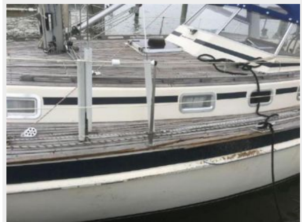
Minor damage from dock piling upon arrival to Rock Hall
