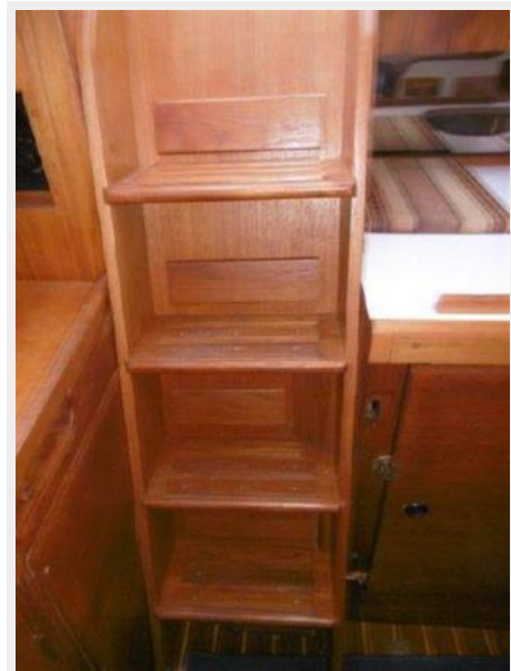
Close up of companionway stairs
