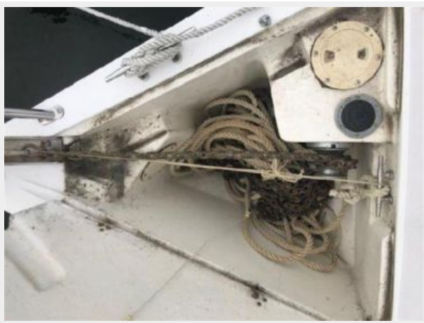
Anchor Well & Windlass
