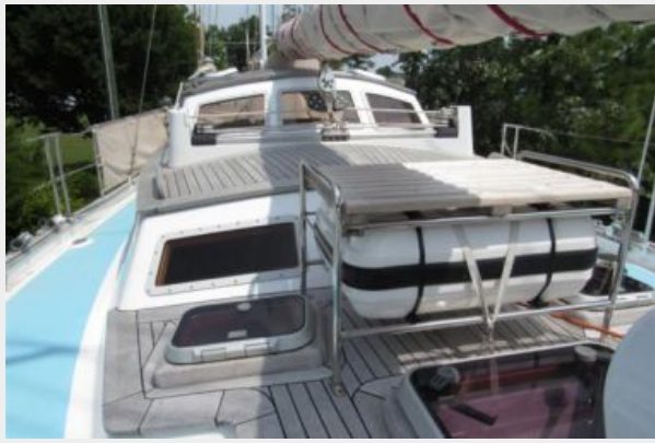
Deck, showing liferaft storage
