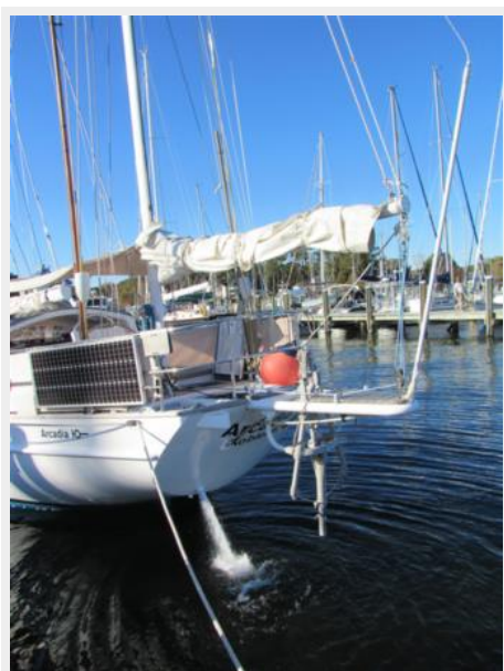
Solar panels, stern and self steering
