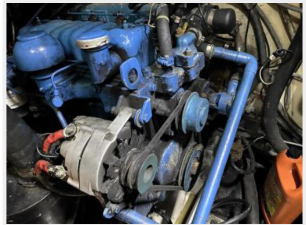
Perkins 4-108 50 HP Diesel engine
