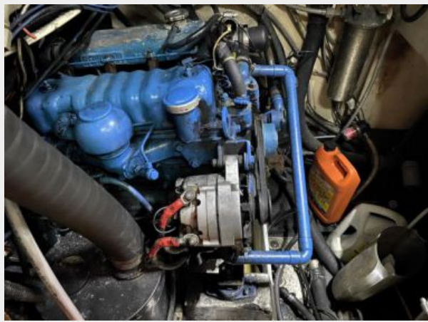
Perkins 4-108 50 HP Diesel engine
