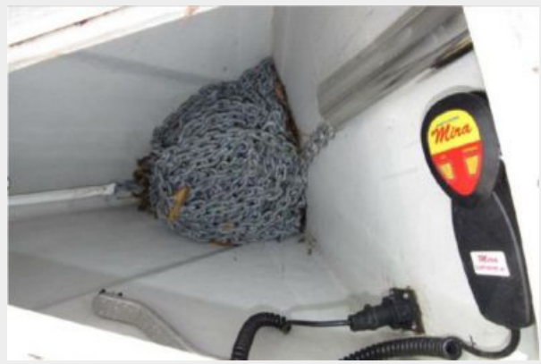
Anchor chain and windlass control
