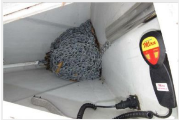
Anchor chain and windlass control
