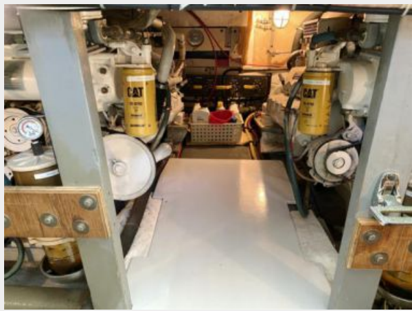
Twin Caterpillar 3208TA engines
