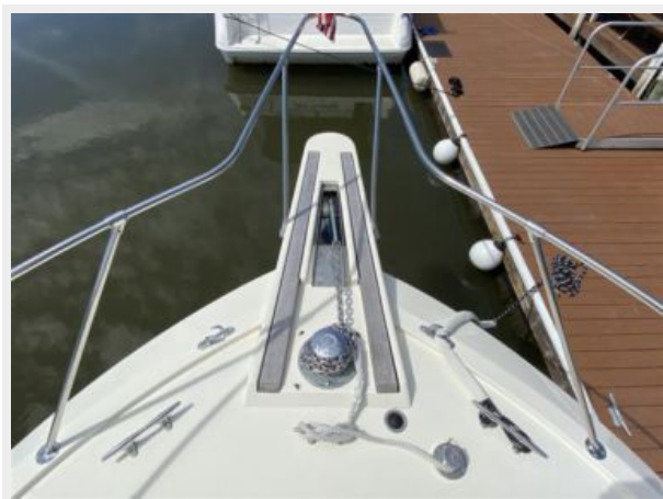
bow pulpit, anchor, windlass
