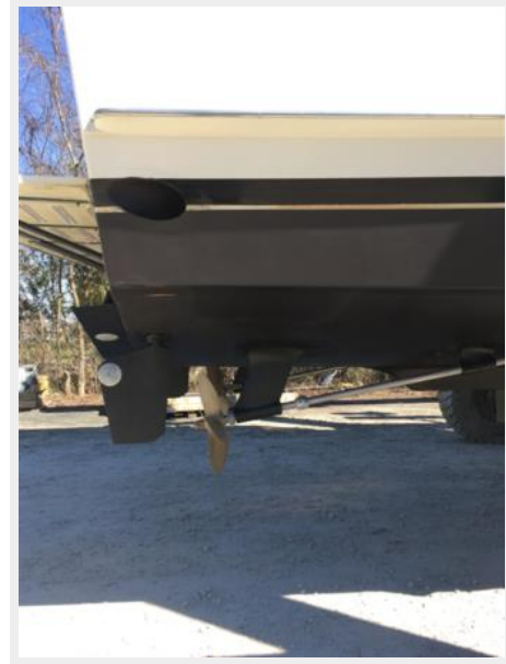
1989 Hatteras 40 DCMY running gear 2020
