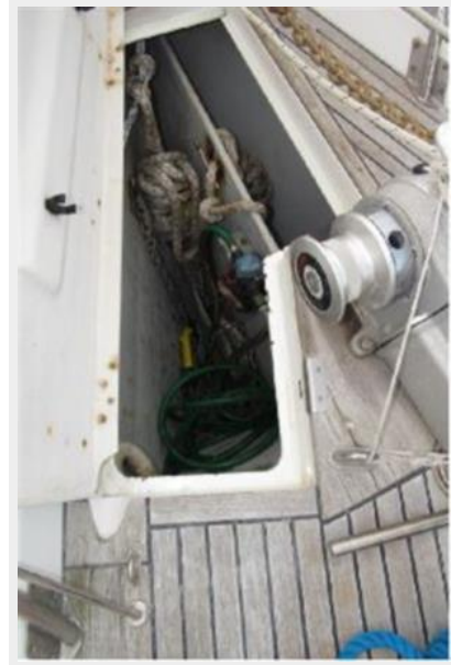
Anchor locker and windlass
