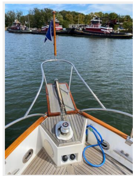
Teak decks and anchor platform, anchor windlass and wash down
