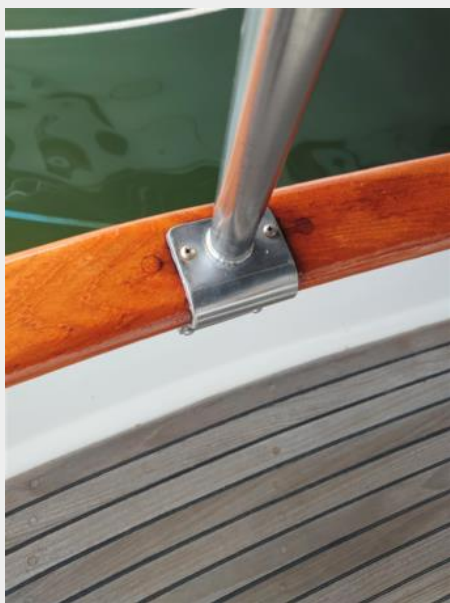
Teak deck and cap rail in very good condition
