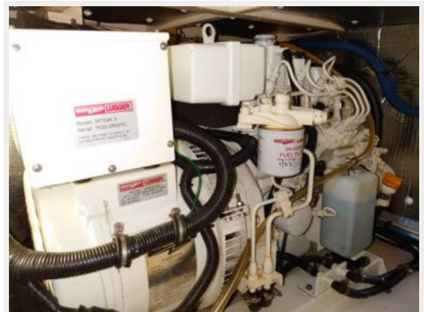
Northern Lights 8 kW generator
