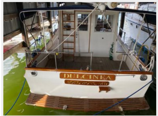
Aft deck with teak sole, fybridge ladder, gelcoated transom, teak swim platform
