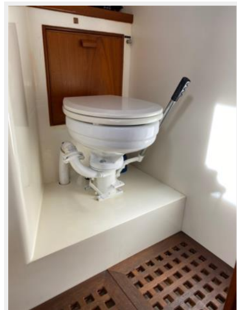
Head with teak cabinet doors and trim, teak grating on sole and in shower
