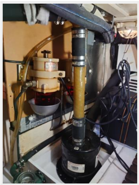
Generator: dual Racor filters, exhaust, muffler
