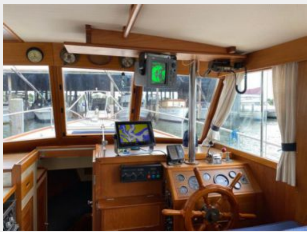
Lower helm station with electronics locker above
