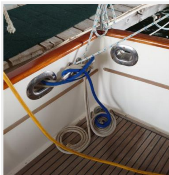
Stainless steel hawse pipes and cleats
