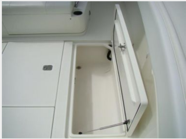
15. Starboard Saddle Box in Cockpit
