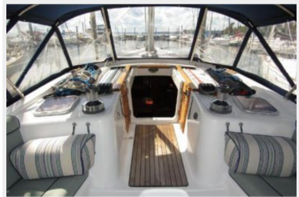
Companionway and cabin top with electric winches and line stoppers
