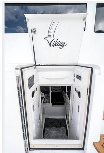
Engine Room Access
