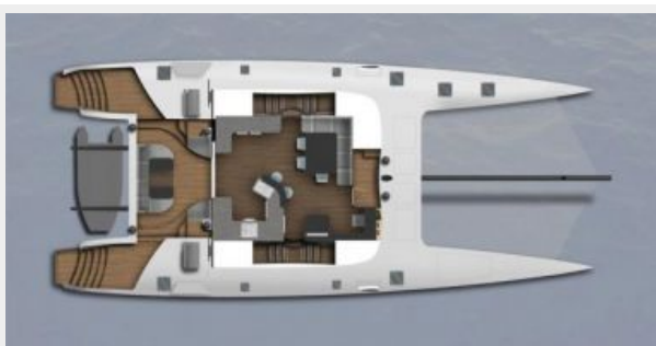
General Arrangement- Main Deck
