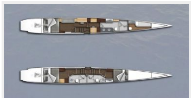
General Arrangement- Below Deck
