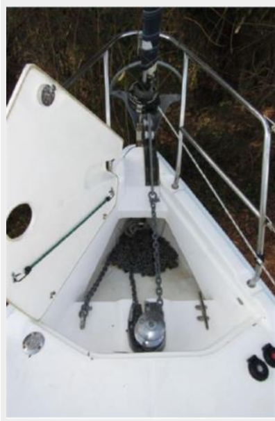
Anchor locker and electric windlass
