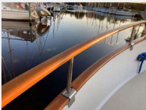
Cap rail, hand rail and connecting s/s stanchion
