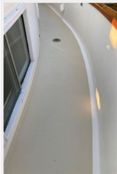
Fibreglass side decks with high bulwarks
