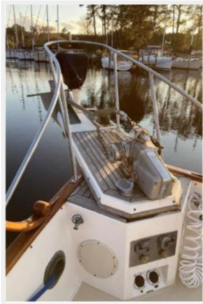
Bowsprit, windlass, shorepower inlets and windlass controls
