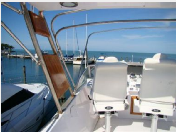
71. Radar Arch + Bimini Top Frame
