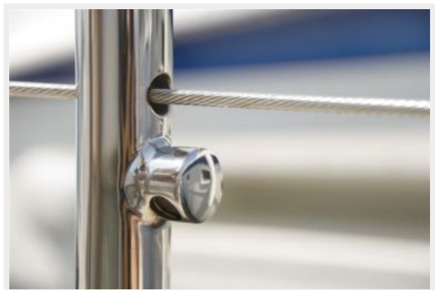
Diesel tank vent in stanchion
