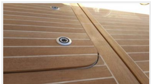
Engine Room Access Hatch
