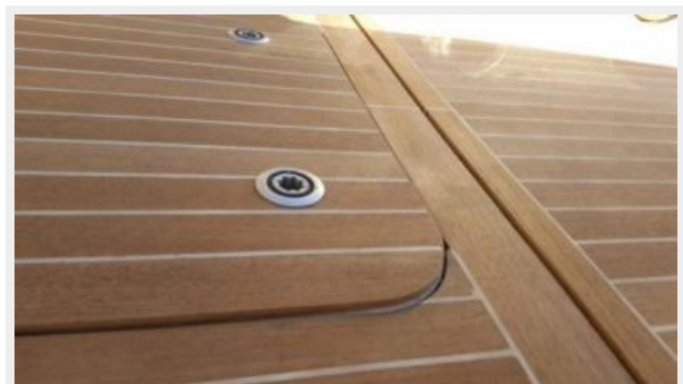
Engine Room Access Hatch
