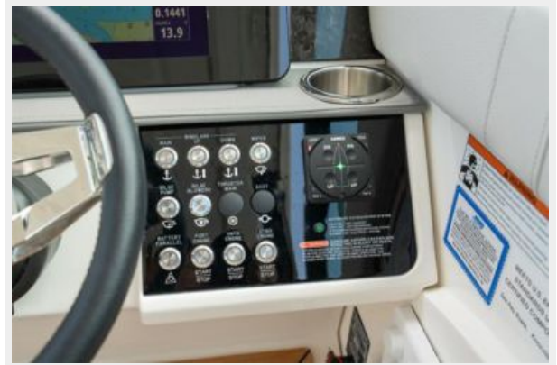
Helm controls/switch panel
