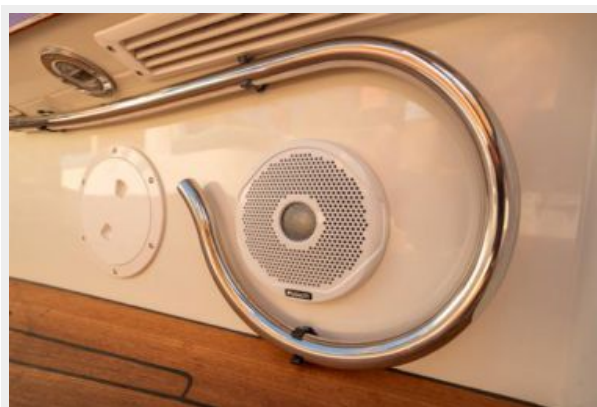
Cockpit speaker with the Bo-Peep stainless steel handrail stored
