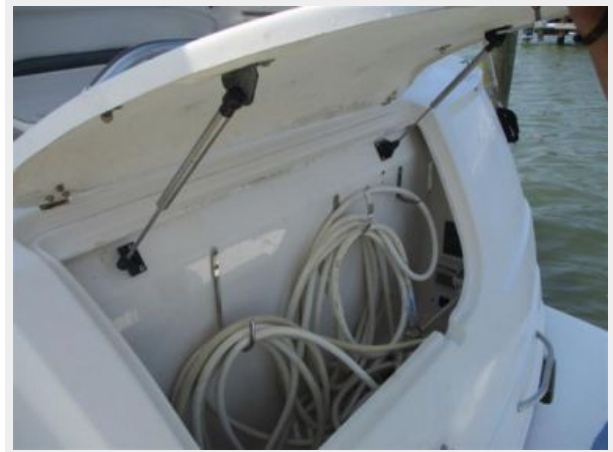
20.30 Amp Power Cord & Storage Aft
