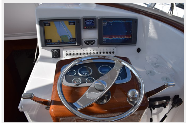
Garmin system with autopilot, CHIRP and radar
