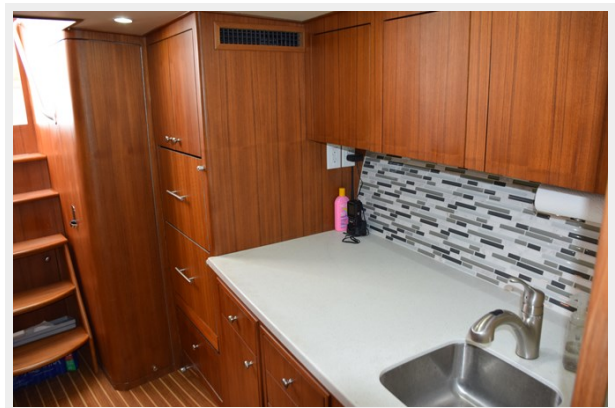
Corian countertops and glass tile backsplash
