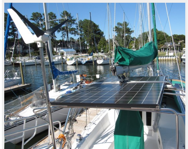
Solar panel & wind generator
