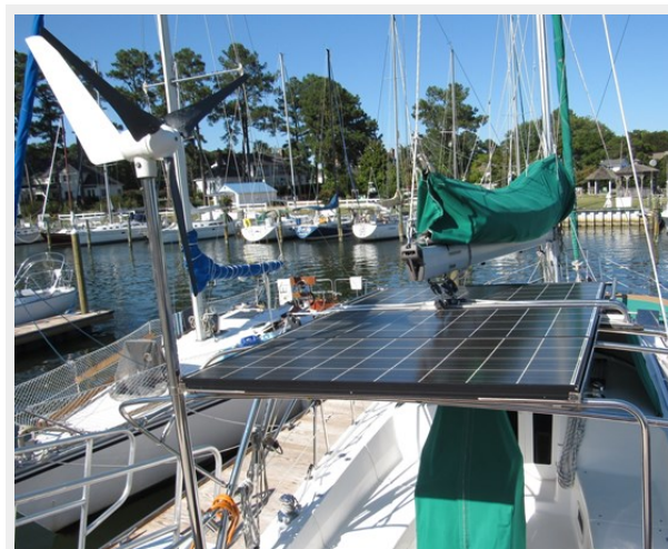
Solar panel & wind generator
