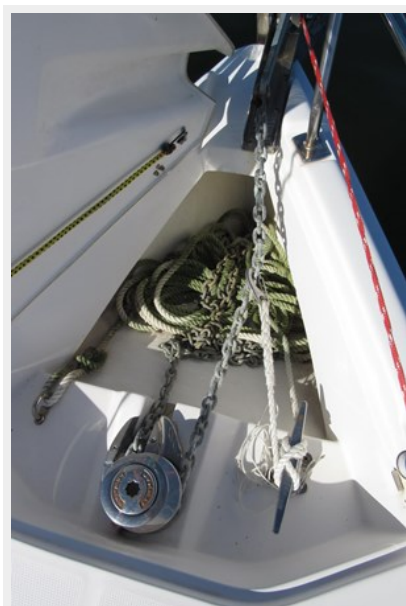
Anchor locker and electric windlass
