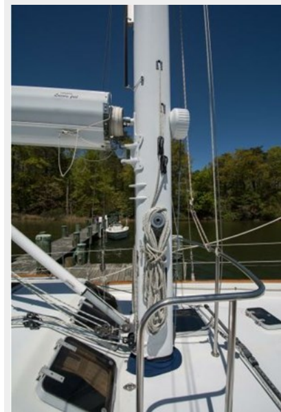
MAST W/ ELECTRIC BOOM FURLING
