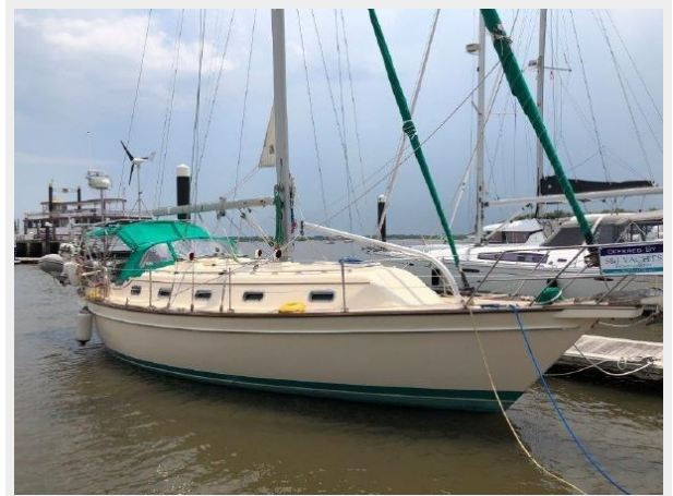
Cutter rig with furling main and head sails
