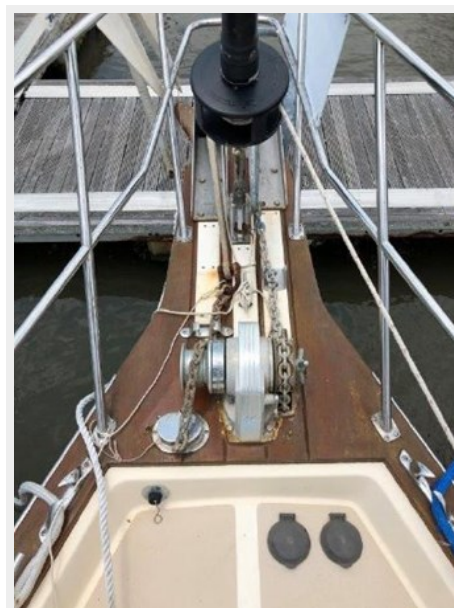
Three anchors, two rollers and a windlass
