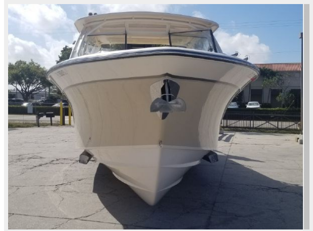
Bow profile w/ anchor & stainless rubrail. SeaV2 hull has a sharp entry angle for great ride
