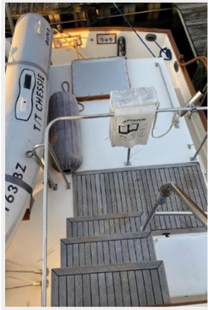
Steps up to flybridge and S/S handrails
