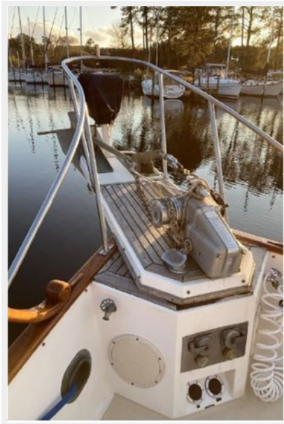
Bowsprit, windlass, shorepower inlets and windlass controls
