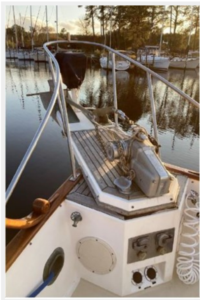
Bowsprit, windlass, shorepower inlets and windlass controls
