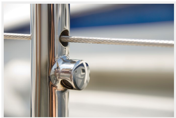
Diesel tank vent in stanchion
