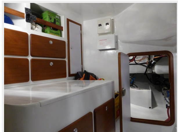
Workbench and access to rudder quadrant
