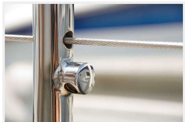
Diesel tank vent in stanchion
