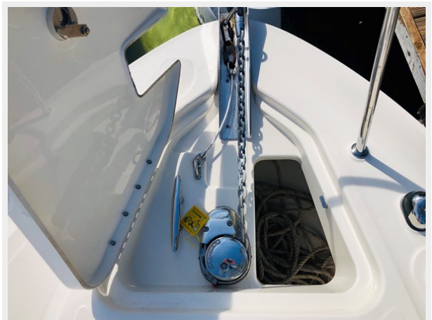
Windlass, Anchor Locker
