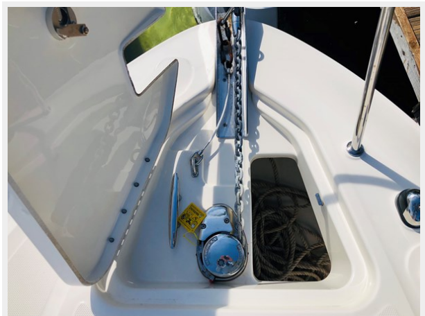
Windlass, Anchor Locker
