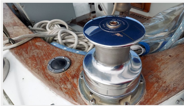
12 Primary winch electric
