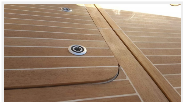
Engine Room Access Hatch
