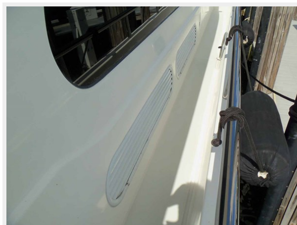
Engine Room Vents
