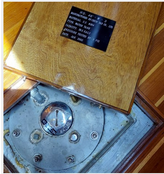
1111 Night Flight Water Tank Starboard
