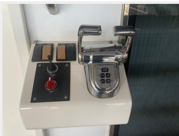
Aft Deck Docking Station
