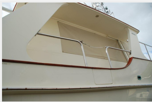
Side Deck Entry Gates
