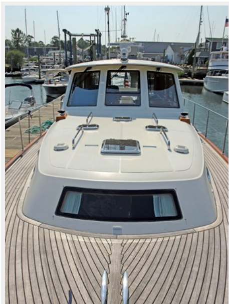
Cabin Trunk, Looking Aft
