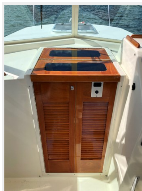
Teak Companionway Hatch and Doors
