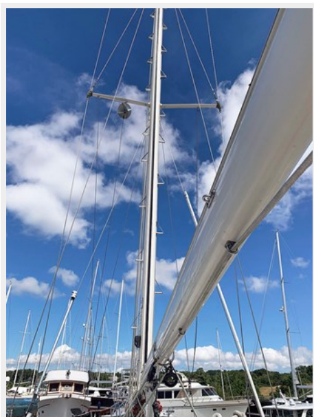
Mast Boom and Rigging
