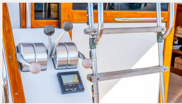
Aft Deck Control Station
