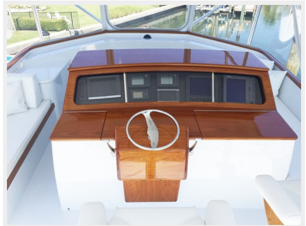
Teak Pod and Console with Single Lever Controls
